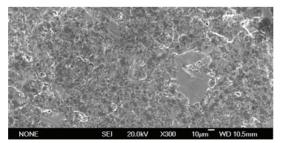
Silicon Carbide aggregates - the key behind crack deflection and exceptional ballistic properties
