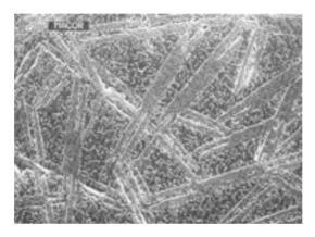
Randomly oriented mica flakes in the microstructure of Macor machinable glass ceramic are the key to its machinability.
